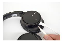
Plug the straight audio jack (either 2.5mm or 3.5mm) into the audio port.
