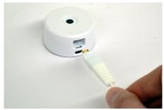
Plug the sensor into a **Powered**Zips Alarm Unit (Single or 4 port). **Note:** The sensor can also be used with S2865 Accessory Boxes,
