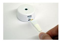
Plug the sensor into a **Powered**Zips Alarm Unit (Single or 4 port). **Note:** The sensor can also be used with S2865 Accessory Boxes,
