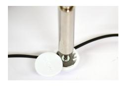
Loosen the screw (do NOT fully remove) inside the retainer using a TT8 bit.
