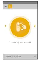
Tap the lock knob with the NFC antenna of the device being used. The lock will unlock and relock within 4 seconds.
