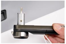
Drill a hole in the drawer face with a 3/16 inch (or 5mm) drill bit.
