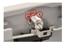
Bend the prongs on the lock washer over the nut to prevent it from loosening.
