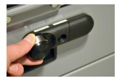
You will have several seconds to turn the knob to unlock and open. If the LED on the lock flashes red before the lock is opened, it will need to be unlocked again.
