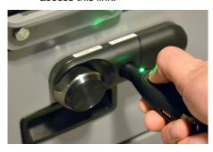
Lock Activation Using OneKEY: Place a charged and coded OneKEY against the lens on the lock and press the button the Key. The LED on the Key and the lock will flash green.
